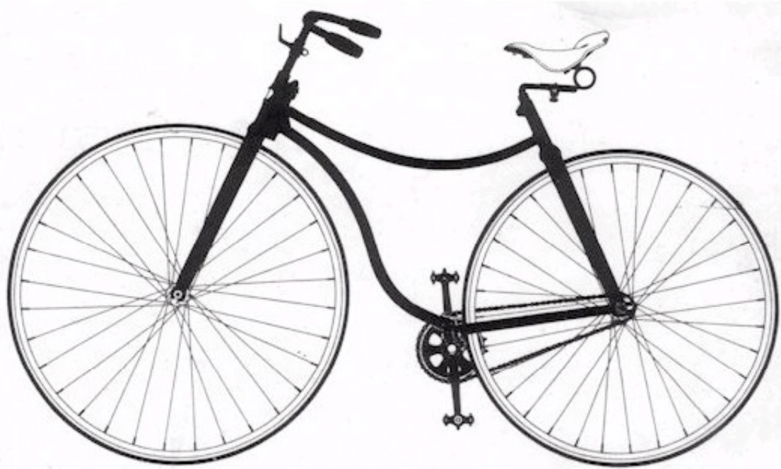
Figure 1.1 John Kemp Starley's Rover 'safety' bicycle (From Heskett's Industrial Design )
